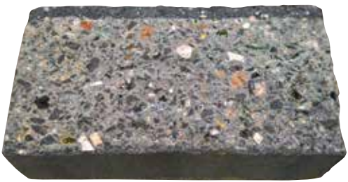
Photo 2. Cross-section of a concrete paving stone with bottom ash aggregate
