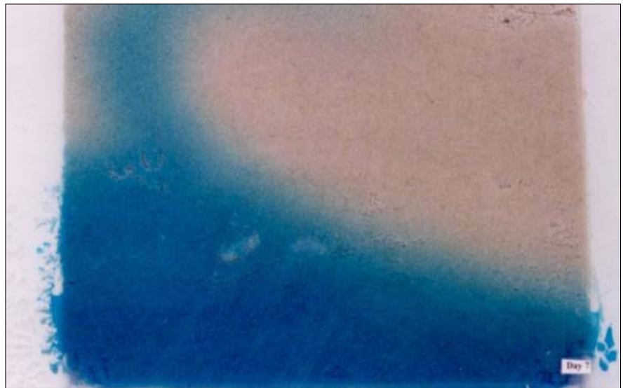
Figure 4: Convective Rise in Solution of Water and Blue Food Dye Induced by a Light Bulb Heating Surrounds by 1°C
