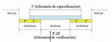
As can be seen in the figure below, there is a T zone (conformance range) in which the result should be found to obtain a conforming concept, however, when the associated uncertainty is applied, there is the possibility that the true value is outside specification, so there is a probability that the result is non-conforming. Considering this risk, you should proceed as follows:
