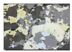
Ores with coarse and fine-grained intergrowths of pyrite, chalcopyrite and sphalerite will pose difficulties during flotation.
