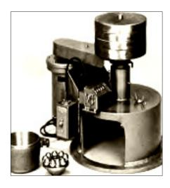
determined sized coal onto a steel plate from a specified height. The shattered pieces are screened and sorted and the mass of each size group is recorded. The percentage of the original sample that shattered into each size grouping is an indicator of the coals friability, and will allow you to estimate the capacity of your coal to resist breakage during handling and shipping at your facility.
