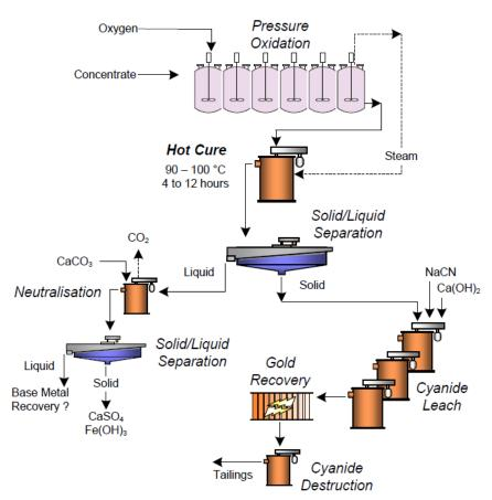
Figure 2 Refractory gold pressure oxidation, hot curing and cyanidation flowsheet Results
