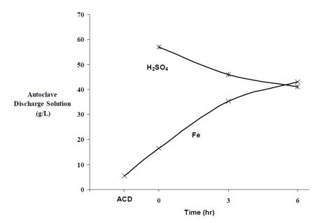
Figure 4 Concentrations of iron and sulphuric acid in solution in the discharge from autoclaving Quimsacocha flotation concentrate, as a function of hot curing time.
