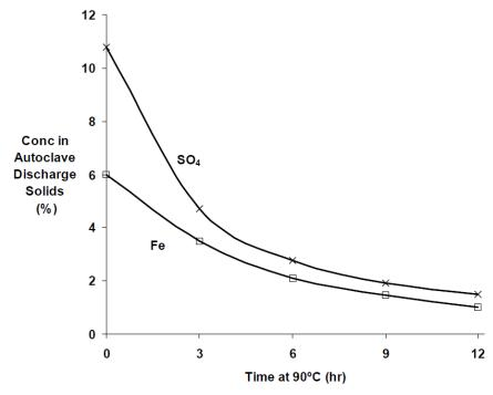
Figure 5 Concentrations of iron and sulphate in the solid residue from autoclaving Pueblo Viejo ore, as a function of hot curing time.
