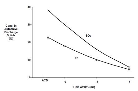
Figure 3 Concentrations of iron and sulphate in the solid residue discharge from autoclaving Quimsacocha flotation concentrate as a function of hot curing time
