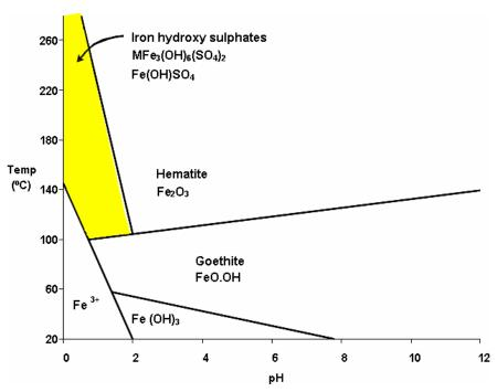
Figure 1 Areas of stability of various compounds in the Fe-S-O system (After Babcan [2])
