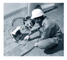
SGS uses pear point flexi probe push rod video inspection systems to inspect pipelines for its internal fractures and blockages etc. It is also incorporated with an universal easy-fit brush skid set to customise the system for use in a wide range of pipe diameters.
