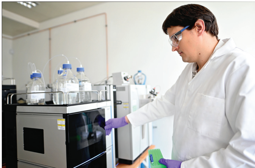
Figure 2. SGS uses liquid chromatography tandem mass spectrometry (LCMSMS) Orbitrap technology to solve complex analytical problems.
