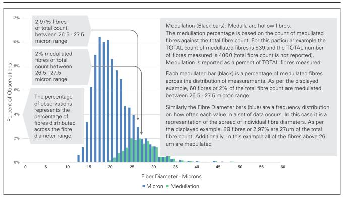
Test Performed According to Method AS/NZS 4492.5:2000
