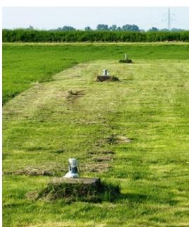
Groundwater monitoring wells at a monitoring test field;
