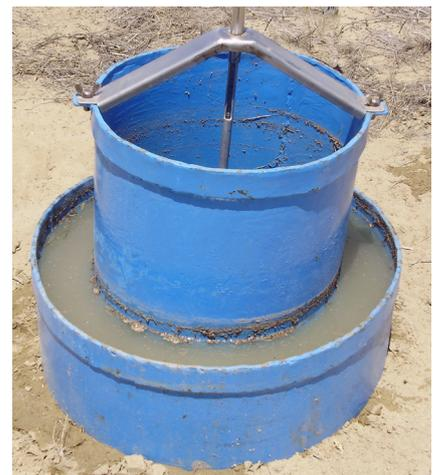
Cylinder infiltrometer double to determine the soil infiltration rate
