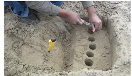
Sampling of undisturbed soil to measure bulk density of soil
