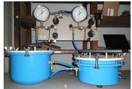
Pot and plate pressure to determine soil moisture curves
