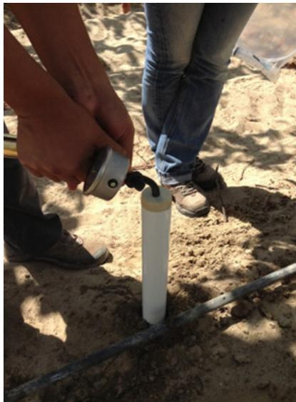
6. Generating a vacuum in the suction probe or Lysimeter to get the sample
