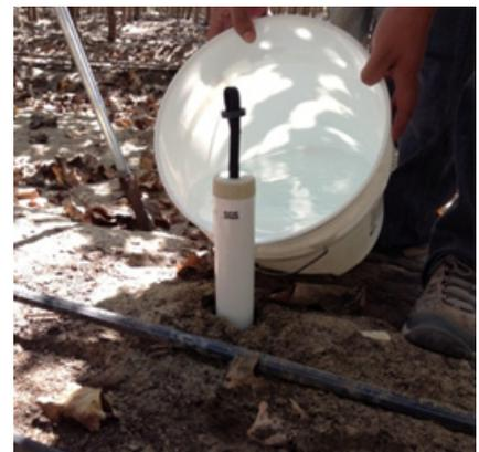
3. Just after the lysimeter or suction probe has been installed in the field, some water has to be put around it to assure it's well placed
