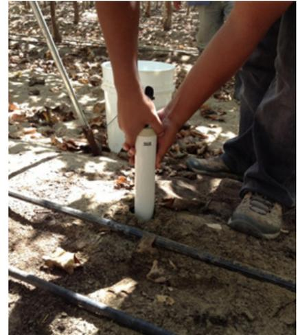
1. Lysimeter or suction probe being installed in the field after the hole was made with the blast hole
