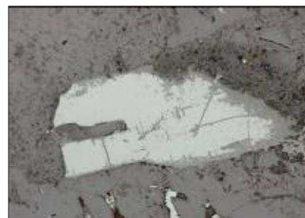
Ferrotapiolite (bright white) (Fe,Mn) (Ta,Nb)2O6 has a different trace element composition (SEM spectrum) from pyrochlore and columbite, and may contain Sn, U, Th and Pb.
