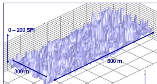
Figure 3 – Hardness surface of a bench
