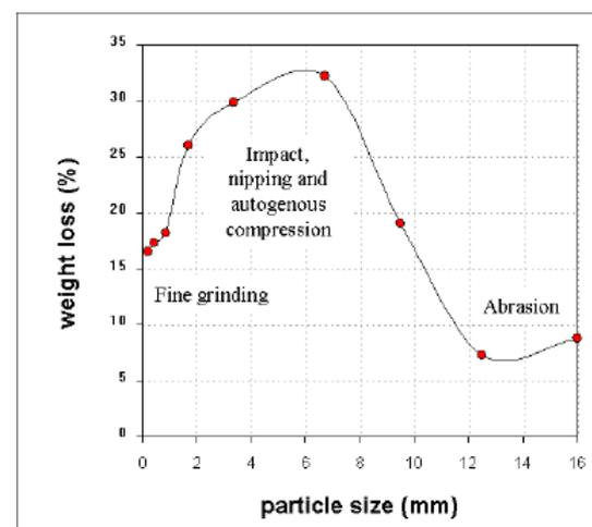
Figure 6 Weight loss by size class in the SPI mill tests with narrow feed size classes. Original ore had an SPI of 62 minutes.
