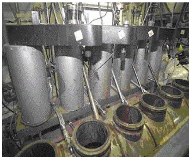
Figure 3 – Continuous Autoclave Agitator Assemblies
